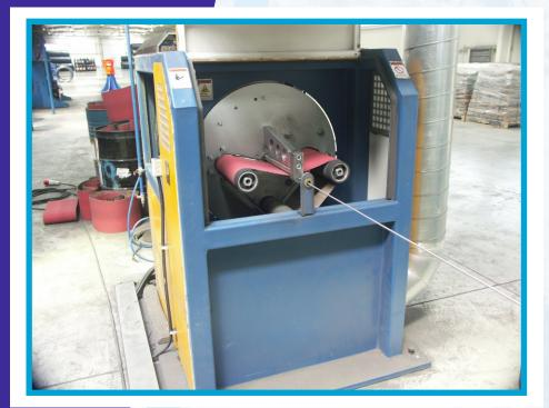
This system enables preparation of wire rod without using acid. This high efficiency system is specially designed to oprate in line with the drawing machine and consists of following eqipment:
